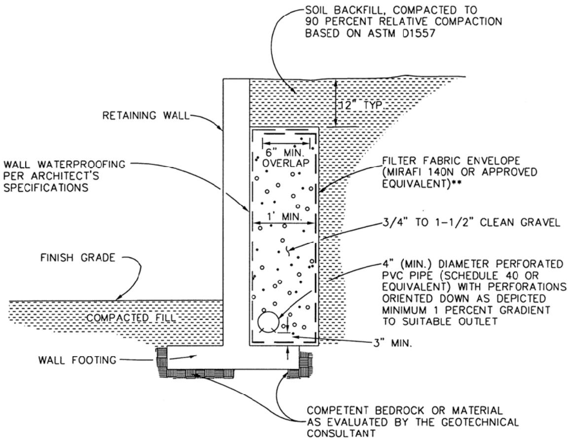
NOTE: UPON REVIEW BY THE GEOTECHNICAL CONSULTANT, COMPOSITE DRAINAGE PRODUCTS SUCH AS MIRADRINK OR J-DRAIN MAY BE USED AS AN ALTERNATIVE TO GRAVEL OR CLASS 2 PERMEABLE MATERIAL. INSTALLATION SHOULD BE PERFORMED IN ACCORDANCE WITH MANUFACTURER'S SPECIFICATIONS.
