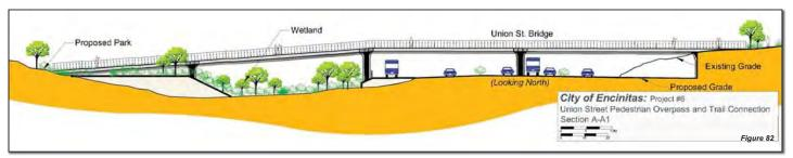
Figure 82 depicts a cross section of the proposed pedestrian overpass connection over I-5 from Union Street to the proposed neighborhood park on the west side of the freeway. Figure 83 is a plan view of the proposed neighborhood park.
