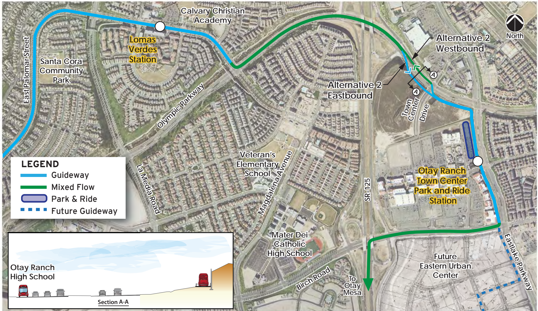
Alternative 2: Olympic Parkway (with an eastbound transit guideway and westbound mixed flow between SR-125 northbound off-ramp and Town Center Drive) with service to Otay Ranch Town Center (ORTC) via a two lane guideway between Town Center Drive and ORTC Station
